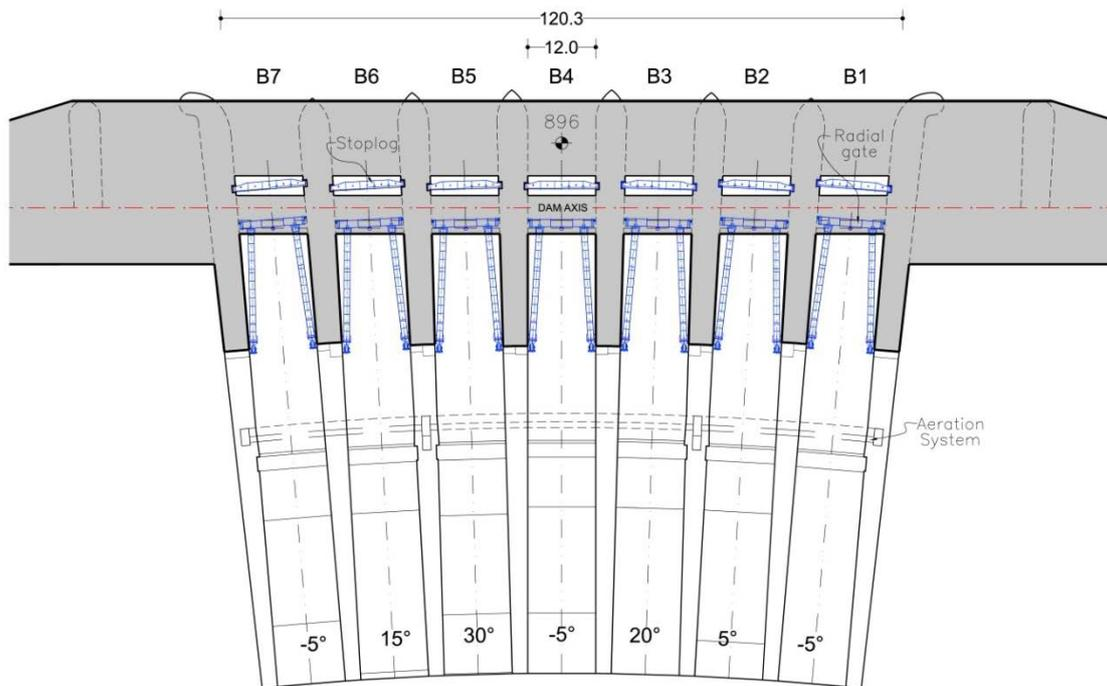
Fig. 2: Spillway plan
