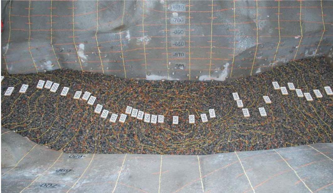
Fig. 8: Physical model with movable bed: bottom of the plunge pool after scour
