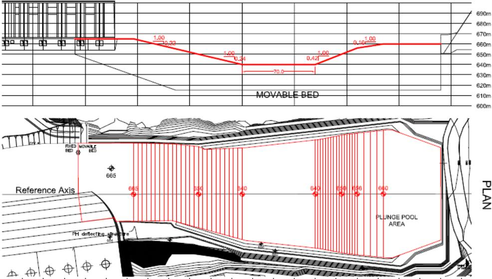
Fig. 7: Plan and profile of the pre-excavated plunge pool
