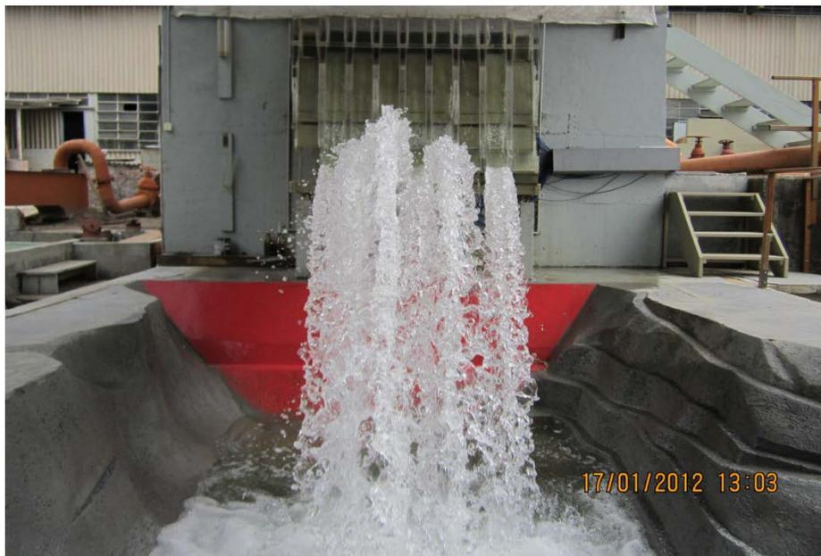
*Fig. 4: Physical model (scale 1:60): test of the design flood with seven chutes*
