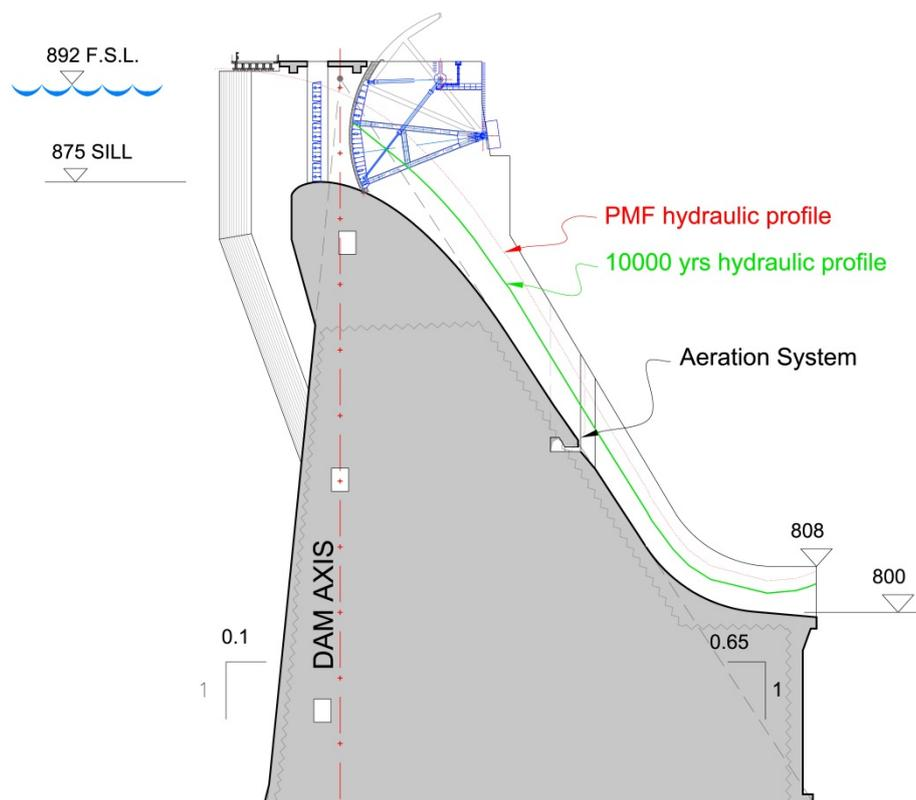
Fig. 3: Spillway, typical section
