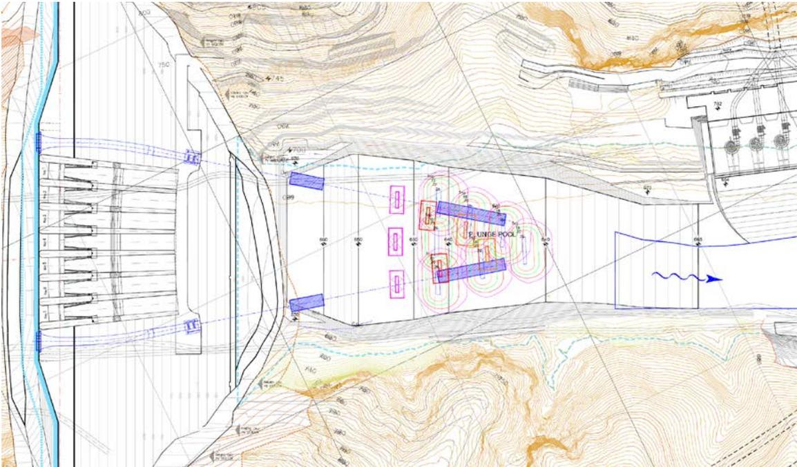
Fig. 6: Layout of the spillway and plunge pool (the impact areas of the spillway jets are indicated in magenta and those of the two middle level outlets in blue).
