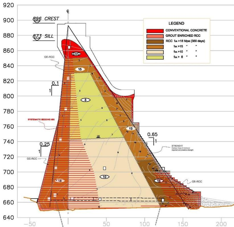
Fig. 8. Gibe III main section (geometry and zoning) at Level 2 design.
