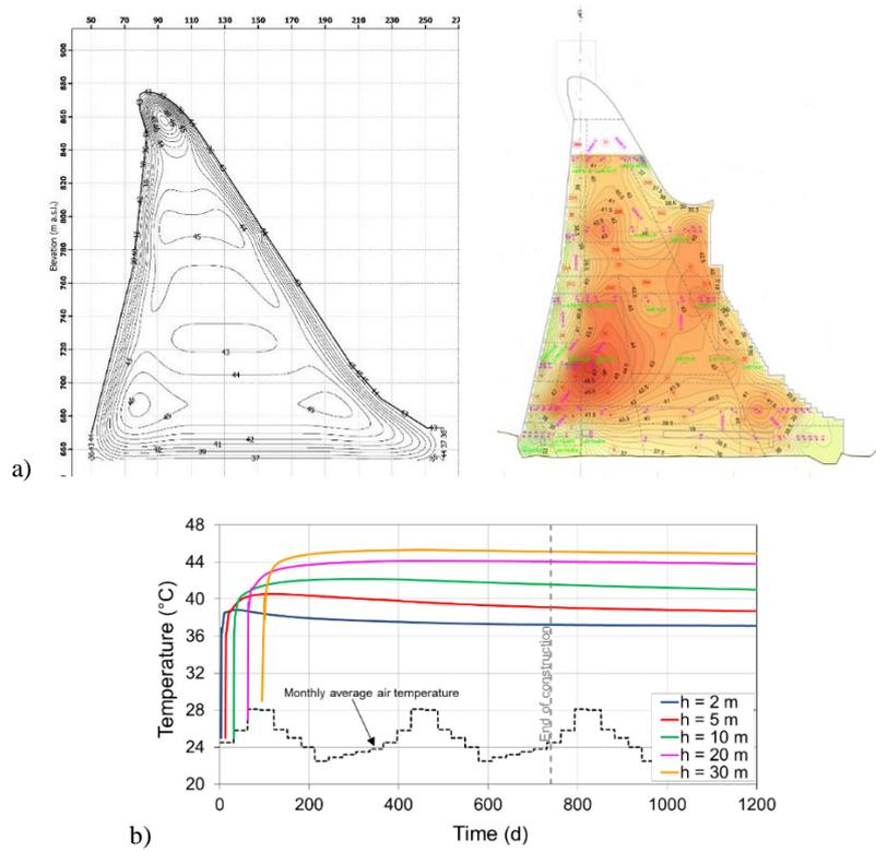
Fig. 7. Thermal analysis, a) Dam temperatures comparison, Design calculation vs. As built; b) RCC temperature history in the dam central zone at different distances from the foundation (h).
