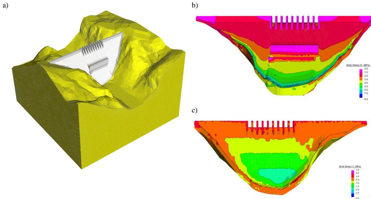
Fig. 6. Dynamic analysis, MCE, a) 3D FEM geometrical model, b) NOC, compressive stress on downstream face, c) NOC, tensile stress on upstream face
