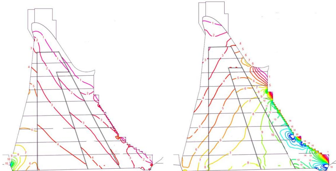
Fig. 3. Minimum required compressive strength; Left: End of construction, Right: Normal operating condition
