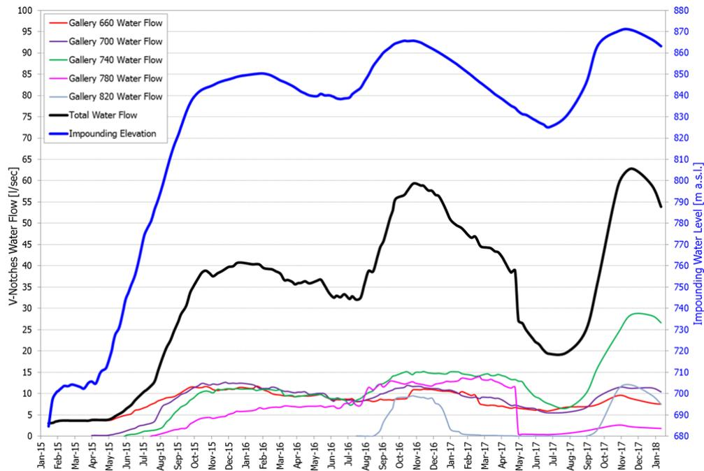
Fig. 11. Overall V-notches discharge and Reservoir Level vs Time
