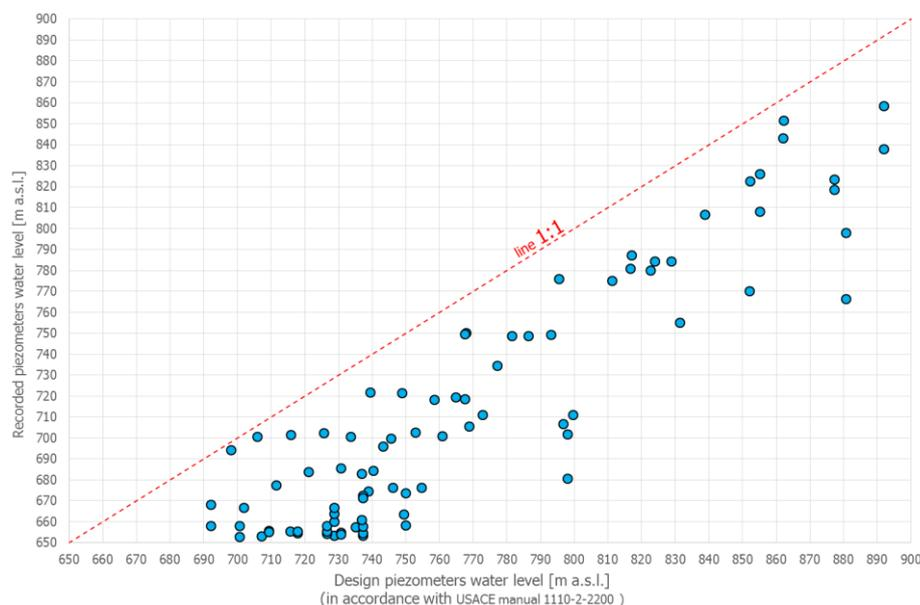
Fig. 10. Piezometers, recorded water level vs. design water level
