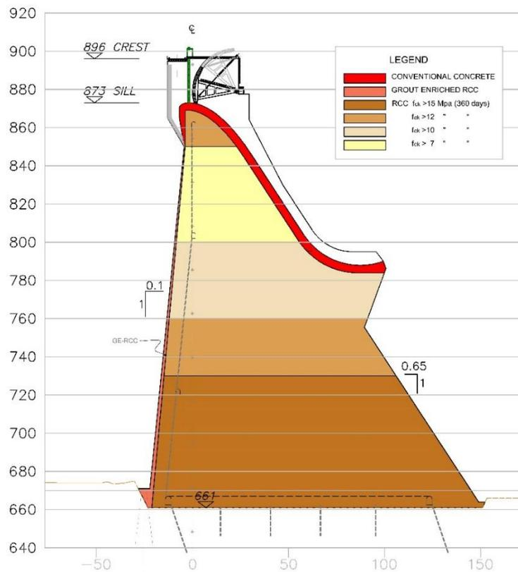
Fig. 2. Gibe III main section (geometry and zoning) at Level 1 design.
