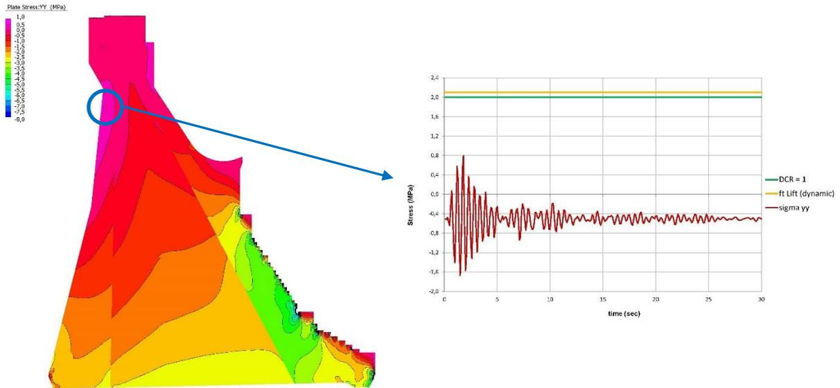
Fig. 4. Dynamic analysis, OBE, Left: maximum vertical tensile stress contour, Right: Tensile stress vs. time (DCR approach)
