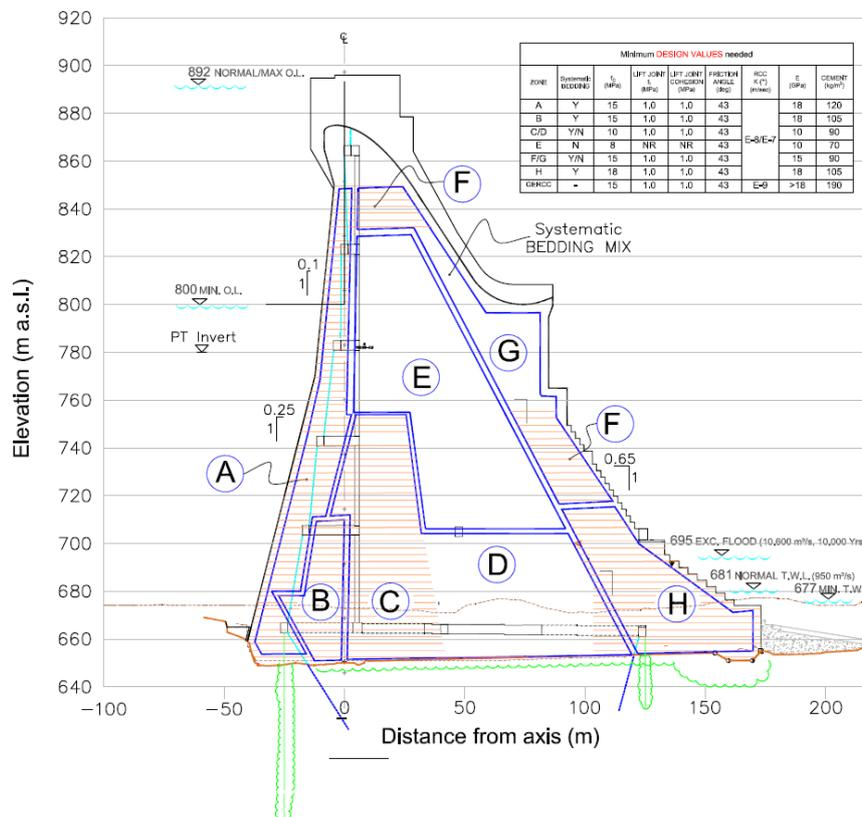
Fig. 9. Gibe III main section, RCC construction zoning
