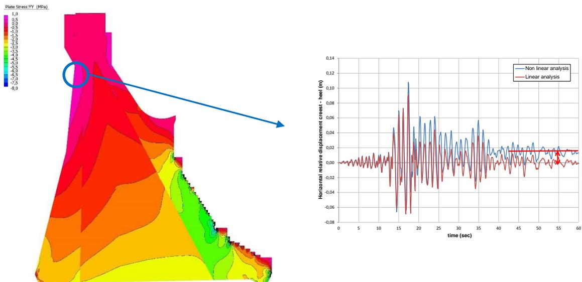
Fig. 5. Dynamic analysis, MCE, Left: maximum vertical tensile stress contour, Right: Displacements vs. time (non linear analysis with multi-cracks approach)
